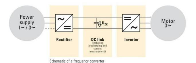
Using a frequency converter in the actuator allows complete control of the motor i.e.: speed and direction of rotation together with torque.
